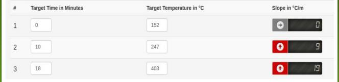
Above Menu is accessed by clicking the icon with 4 lines next to the eye you can now adjust Time and Temperatures here using keyboard this also displays slope in minutes.
