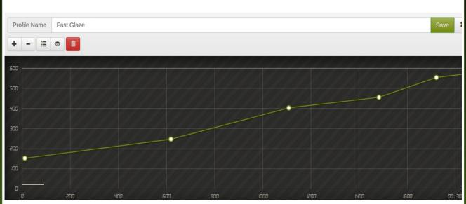
Above the Graph Plotting, you can program your controller just using the graph each white dot added is another a stage click and drag these.(Touch not working on this yet) Temperature is on the Displayed Left
