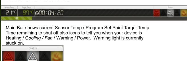
Main Bar shows Heating / Cooling / Fan / Warning / Power.
